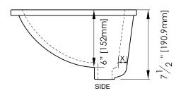
x = 1 1/8" [28.5mm] Back of drain hole to inside back of basin
